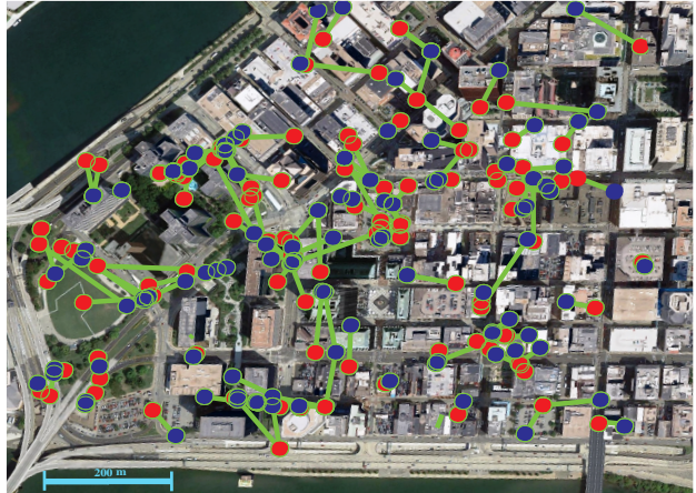
Figure 1. The user-specified GPS-tags (blue) of about 100 images from Pittsburgh along with their correct GPS-locations (red). The green line connects the user-specified location to the ground truth. Significant inaccuracies in the GPS labels can be observed. In this paper, we propose a robust method for refining the GPS-tags.
